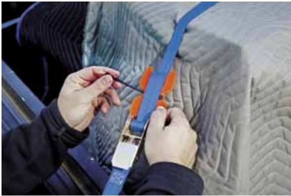
3. Wind rubber cord around strap and snap into cord hook
