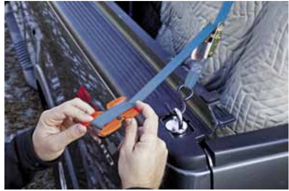
2. Flip Strap-Loc end over end to wrap up excess strap
